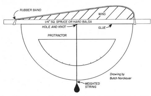
Inexpensive wing incidence meter used by Frank Deis and Hugh Heater. See text for the details.
